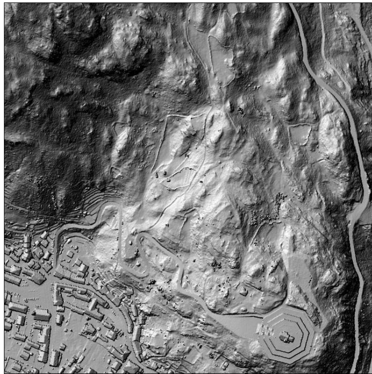
Figure 8: Filtered elevations reveal some of the features connected with past human activity. Terraces, stone walls, entrenchments, plateaus, trenches ... can be observed and mapped. To reveal as many details as possible vegetation filtering was not extensive and some points belonging to vegetation remained in the relief.
